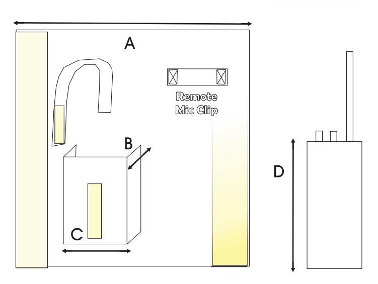
NOTE: For measurement A. Take a piece of string and wrap it around the upright. Then measure that length with a ruler or tape measure. Yellow areas mark were velcro is placed.
